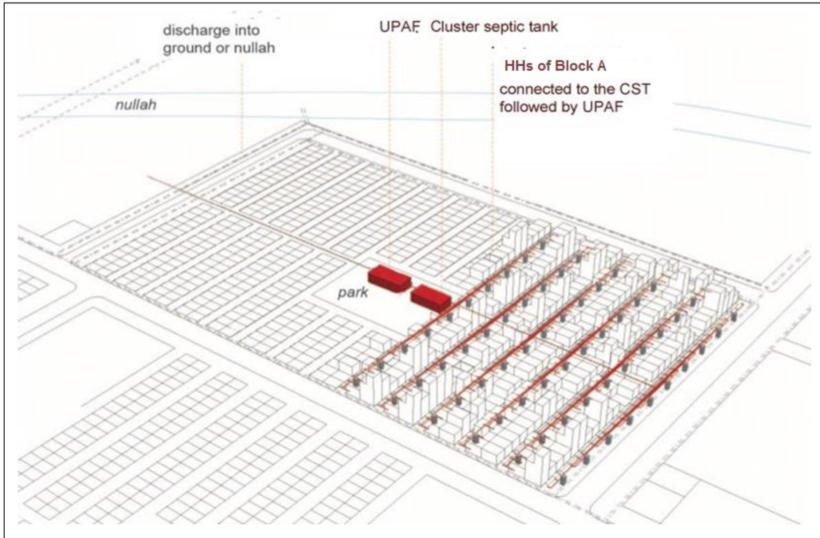
Diagram showing sewer network connected to treatment units (For 322 HHs of A block)
